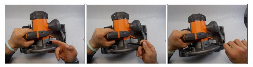
• Pull out the Spindle Lock.
