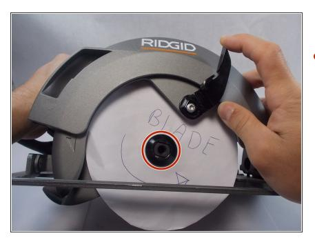
Release the spindle lock and remove the outer flange by lifting it off the output shaft.
