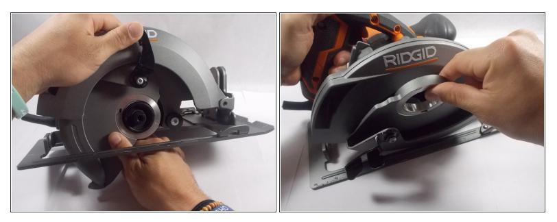
• Remove the lower blade guard after removing the washer.
