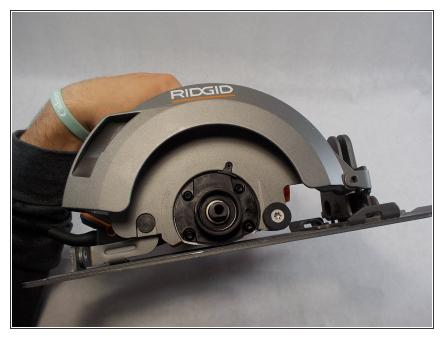
• Leave the rubber dust cover below the removed screw.
