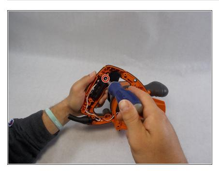
Using a phillips head screwdriver remove the (M4 x 12 mm) screw holding the switch in place.
