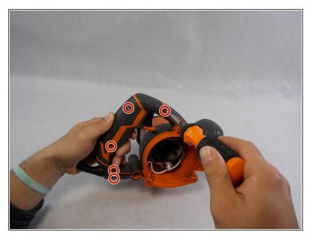
• Remove 5 Torx 20 (#8-16 x 5/8 in.) screws from the outer handle.
