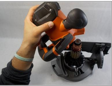
• The motor housing assembly can now be removed from the rest of the saw.
