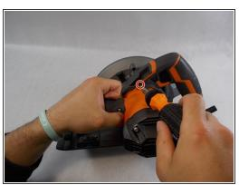
• Use a T25 Torx screwdriver to remove 3 (M5 x 58 mm) screws.
