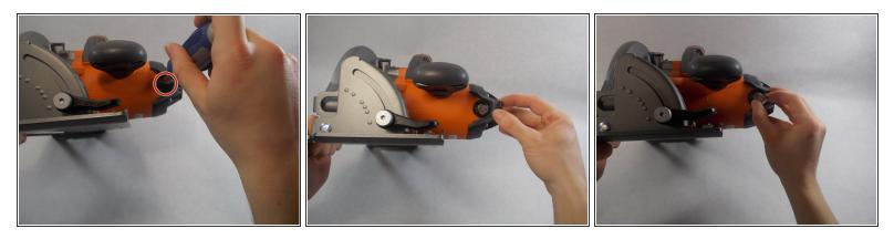
• Remove the brush assembly with a flat head screwdriver.
