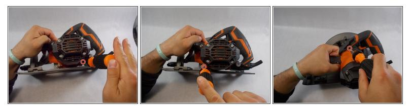
Use a T25 Torx screwdriver to remove 3 (M5 x 58 mm) screws.
