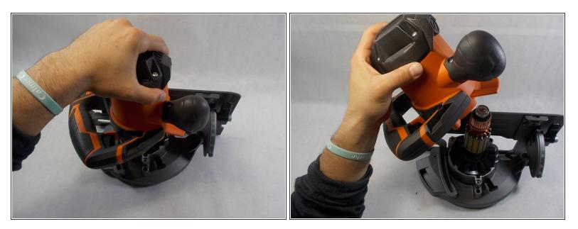
• The motor housing assembly can now be removed from the rest of the saw.
