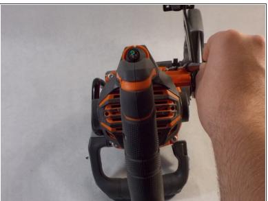
Using the T20 Torx Screwdriver, remove the four 10 cm screws that attaches the main housing assembly to the gear box.
