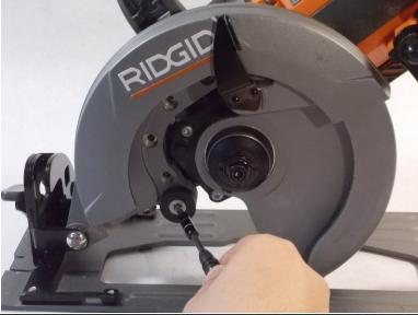
Using the T50 Torx Screwdriver, remove the one 5/10 screw that attach to the gear box.
