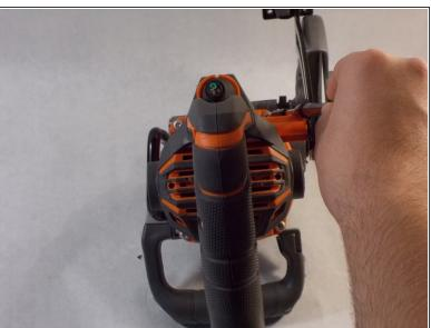
Using the T20 Torx Screwdriver, remove the four 10 cm screws that attaches the main housing assembly to the gear box.
