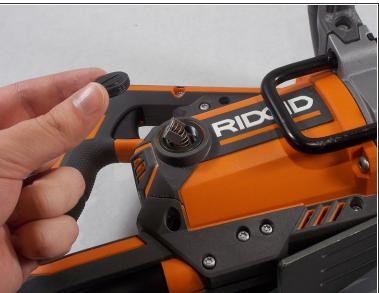
Using a flathead screwdriver, remove the motor brush cap from the main housing assembly.
