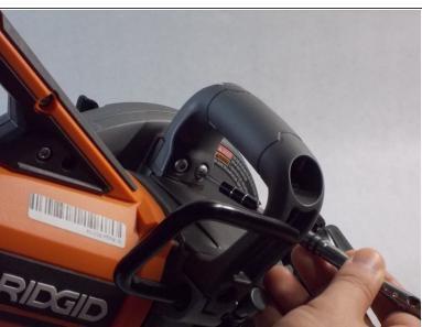
Using the T20 Torx Screwdriver, remove the two 4/10 cm screws that attach to the handle of the device.
