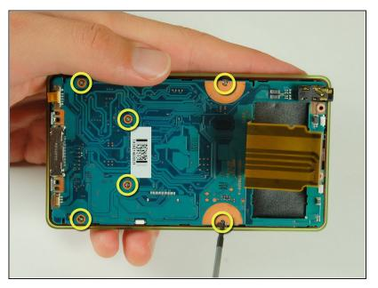
With a Philips #00 screwdriver, remove the six 4.2 mm screws that attach the logic board to the front plate.
