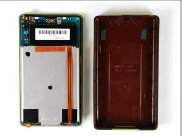
• Turn the Zune over so the screen faces downward. This will ensure the battery does not fall out and pull on the cable.
