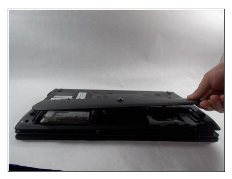
Lift up the back cover of the device, you may need to use a spudger to assist.
