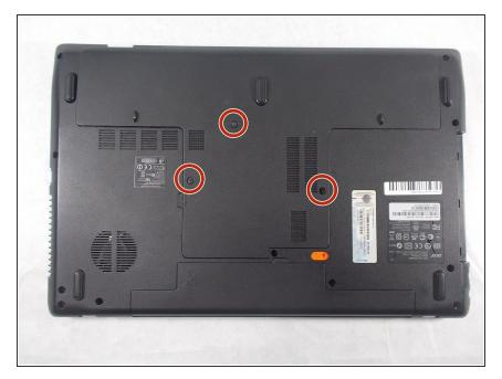
Remove three 60mm Phillips #00 screws that are holding the bottom cover in place.
