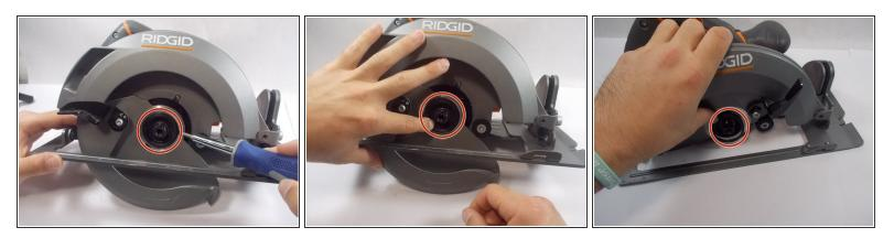
• Remove the external retaining ring with a screwdriver by expanding it and then prying it out.
