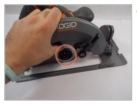
After removing the external retaining ring, remove (OD50 x ID42 x 0.8t) washer.
