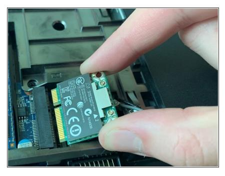
• Use your fingers to pull out the WLAN module as shown.
