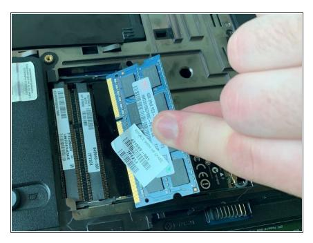
• Directly pull out the memory module as shown.
