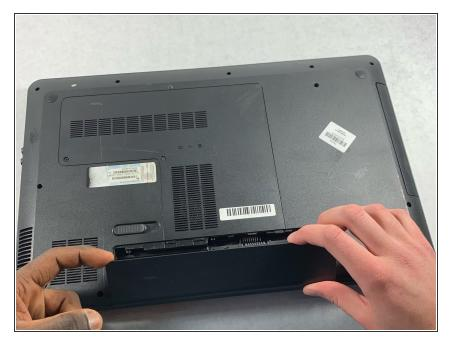
While pushing the switch, lift the battery by the side closest to the switch up and away from the laptop.
