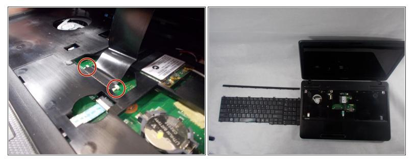
• With the keyboard resting up, pull the tabs to disconnect the cable from the laptop.
