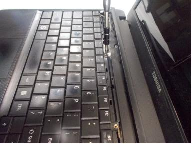
Using a phillips head screwdriver, unscrew each of the four screws.
