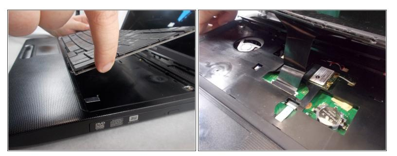
Gradually lift the keyboard up, it will reveal the connector cable.
