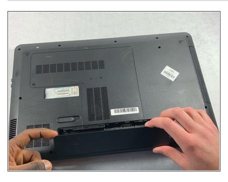
While pushing the switch, lift the battery by the side closest to the switch up and away from the laptop.
