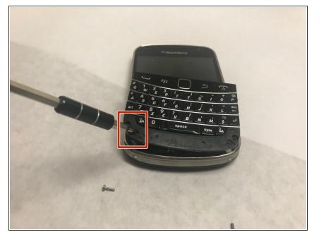
• Now lever the keyboard up using the screwdriver in the indicated hole.
