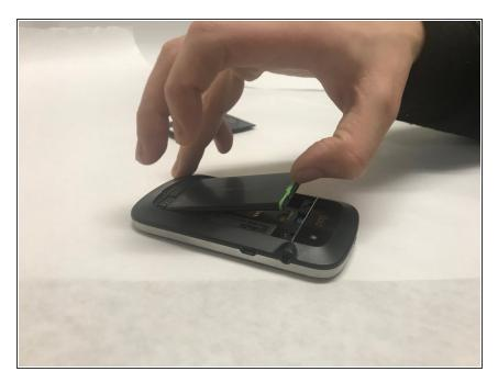
• Lift the edge of battery with the green stripe upward to remove battery.
