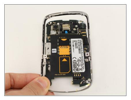
• Lift the midframe, which contains the power/volume buttons, off of the motherboard and screen.
