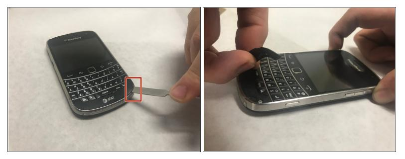
• Lift the bezel at the bottom of the phone up and peel it away from the phone.
