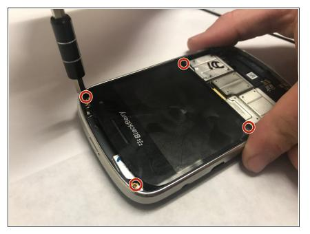
Using the T5 Torx Screwdriver, remove the four torx screws that are located on the bottom half of the device
