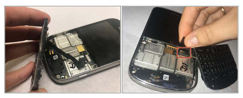
• The keyboard is attached via a ribbon cable. Pull the cable up to remove the keyboard.
