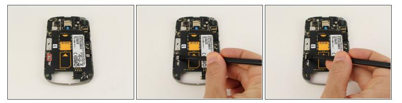
Use the black nylon spudger to pop the press fit connector up from the lower left corner of the motherboard.
