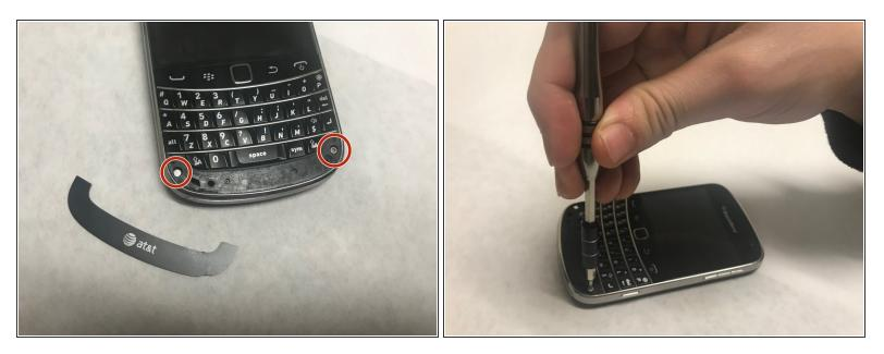
• Remove the two exposed screws using the T5 Torx screwdriver.
