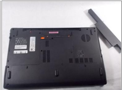
Remove the battery and then pull it out of the device.
