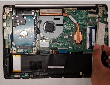
Lift the perforated metal cover up from the motherboard to expose the memory cards.
