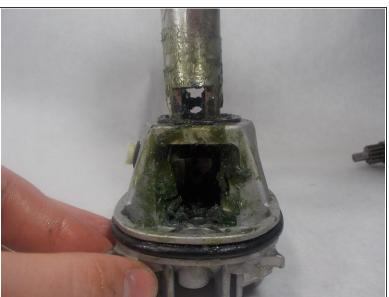
Remove the metal piston from the diaphragm assembly.
