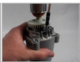
Remove the two 11.5mm T10 Torx screws shown in red.
