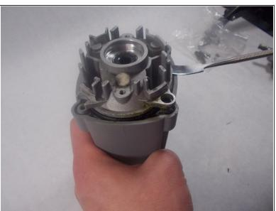
Using a metal spudger, pry the diaphgram assembly out of the gear case.
