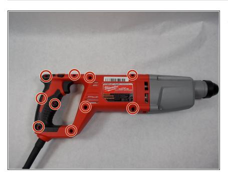
Remove the ten 19mm T20 Torx screws shown in red.
