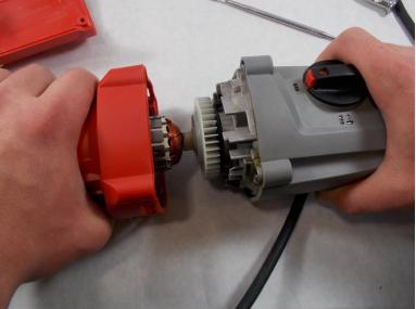
Pull the front portion of the tool out from the motor housing.
