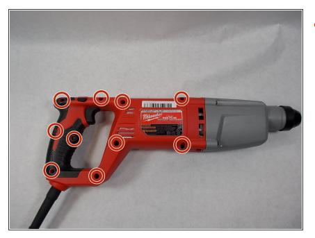
Remove the ten 19mm T20 Torx screws shown in red.
