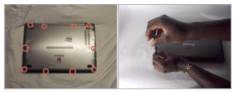
• Remove the ten 5 mm screws that hold the backplate using the Phillips #000 screwdriver.
