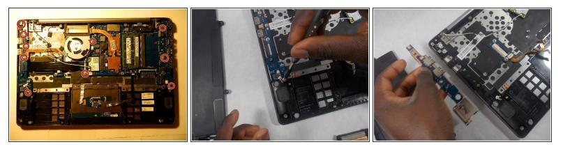
Remove the screws of the motherboard to disconnect the motherboard from the speakers using a Phillips #0 screwdriver.
