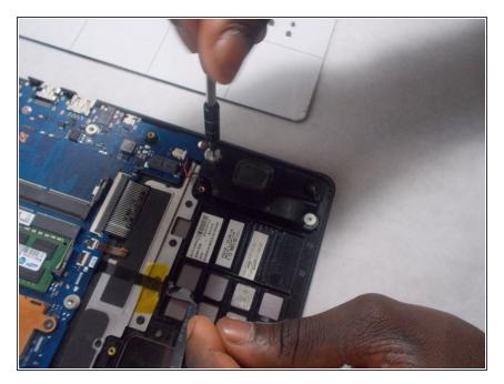
• Remove the 4 mm screw with the Phillips #000 screwdriver and remove the speaker.
