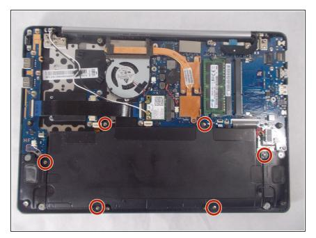
Remove the six 5mm screws that hold the battery by using the Phillips #0 screwdriver.
