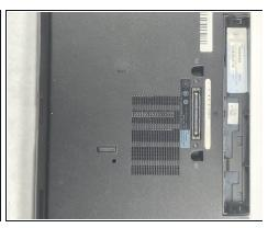
Slide latches out to unlock and remove battery.
