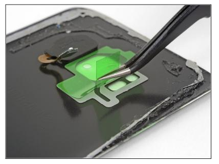
• Peel the green backing away from the adhesive strip. Make sure the adhesive does not come off of the glass with the backing.
