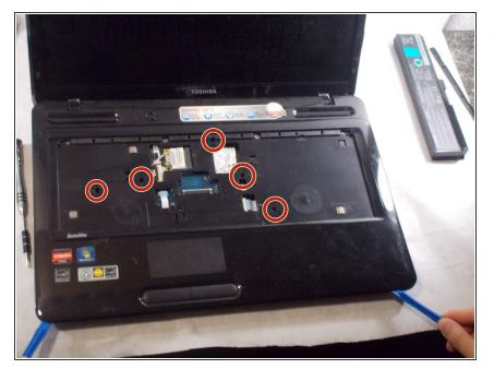
Turn device over so you are looking at the top of the device. Then, remove these five 5mm screws from under the keyboard.
