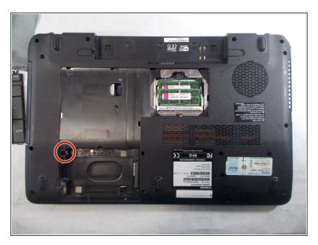
• With the cover removed, locate and remove single screw with Phillips head #1 screwdriver.
