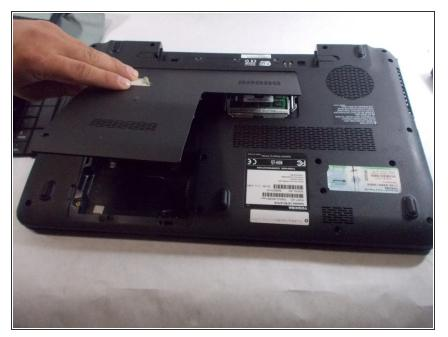
• Lift the removal tab upward, you will hear the clips that hold the tab release. Move in a clockwise direction releasing the remaining clips. Once all clips are released, remove the cover.
