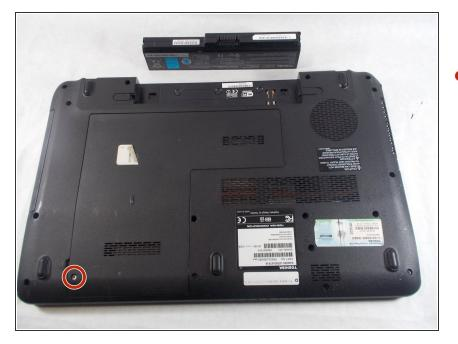
With the device flipped on its back, identify the screw shown and remove with Phillips head #1 screwdriver.
