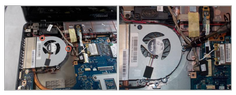
• Locate and remove the two 5mm screws using the screwdriver.
