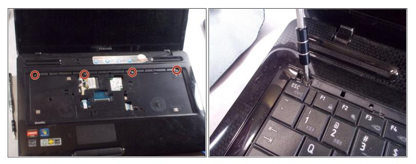
• With the screws exposed, grab your Phillips #1 screwdriver and remove the four 4 mm screws.
