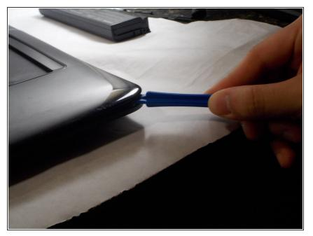
• Pry from under the top case housing along the perimeter of the device with the plastic opening tool.
