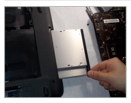
Pull the now revealed part of the disk drive in the direction shown until the disk drive is released.
