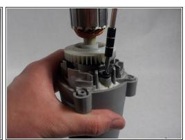
Remove the two 11.5mm T10 Torx screws shown in red.
