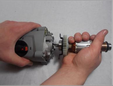
Pull the 120V armature assembly out of the diaphragm assembly.
