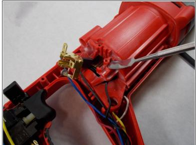
Using a metal spudger, pry off each brush holder.
