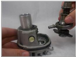
Now pull the reduction gear assembly up and out of the diaphragm.
