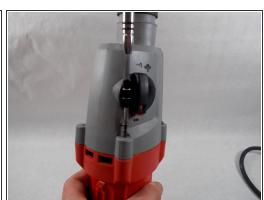
Remove the four 37mm T20 Torx screws shown in red.
