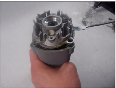
Using a metal spudger, pry the diaphgram assembly out of the gear case.
