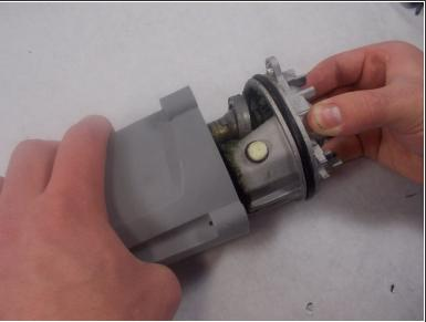
Now that you have loosened the diaphragm, you can now pull it out of the gear case.
