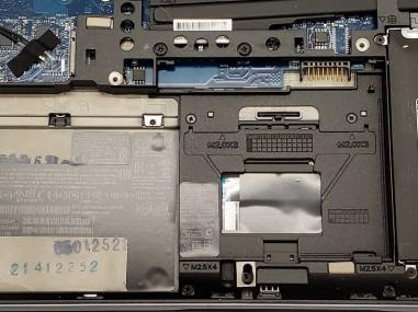
Lift tab and remove battery.
