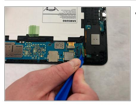
Disconnect the strip from the motherboard with the iFixit opening tool.
