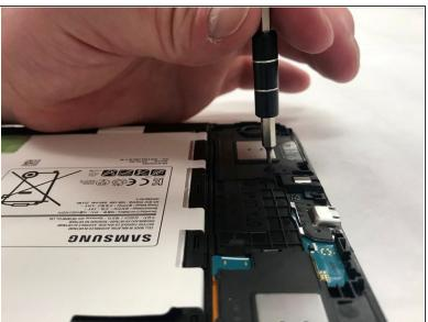
Remove five 2.8 mm screws using the Phillips #000 screwdriver.
