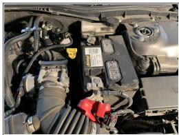
Locate the battery near the top right side of the car if looking at it from the front, and also pull back the red rubber guard covering the positive terminal as shown below.
