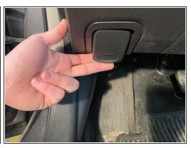
• In order to access the car's battery, the hood must first be opened. To open the hood, begin by pulling the hood release latch.
