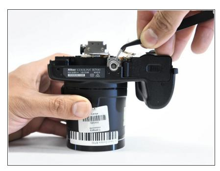
Remove the tripod mount from it's slot.
