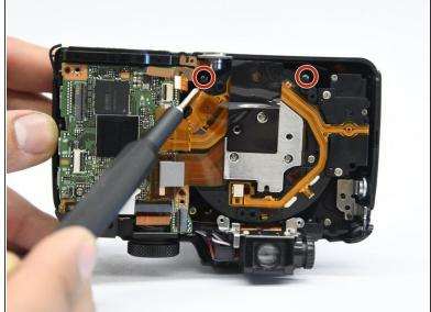
• Use the Phillips screwdriver to remove the four 6 mm screw that hold on the bracket housing.
