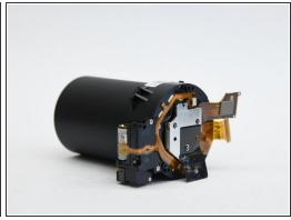
Now you just have to slide the lens assembly out of the housing.
