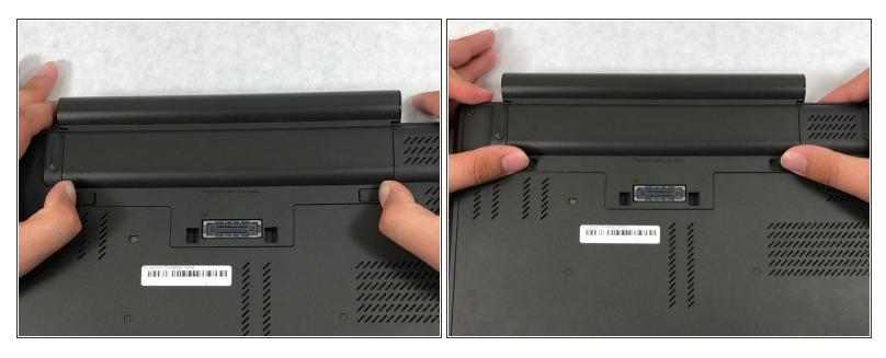
Slide the battery latches to the unlocked position.
