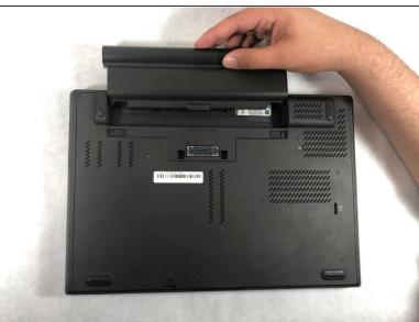
Slide the battery pack out of the battery slot.
