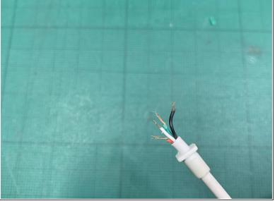
Cut the wires to expose enough coper to be able to solder them to the connectors. Try to get all four to the same length.
