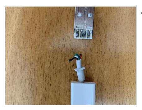
before separating the parts pay attention to the colours of the wires, which ones goes to which connector. Always a good idea to take a picture. On this apple USB cable (30-pin first generation to USB) it goes, left ro right, black,white,green,red.
