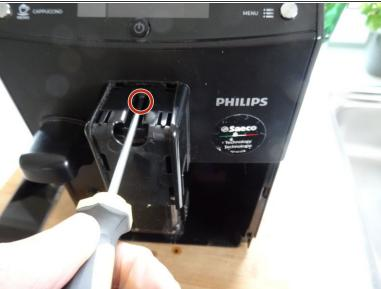
Remove the Torx T10 screw at the top edge of the coffee dispensing spout.
