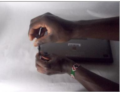
Remove the ten 5 mm screws that hold the backplate using the Phillips #000 screwdriver.
