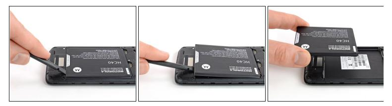
• Use a finger or spudger to lever the battery out of its recess and remove it.
