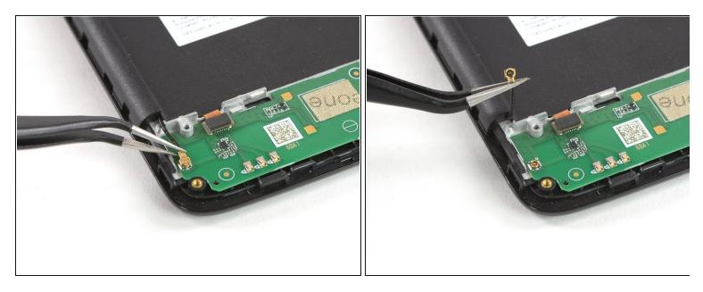
• Use a pair of tweezers to disconnect the antenna cable on the left of the daughterboard.
