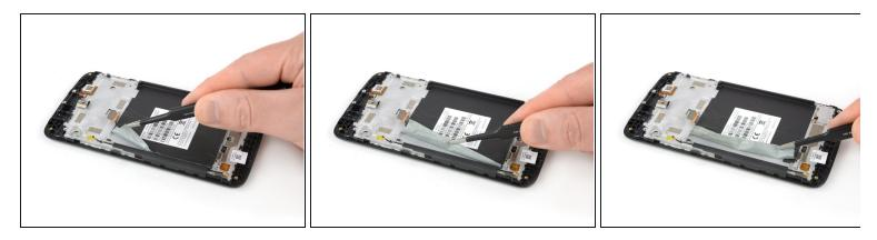
• Use a pair of tweezers to peel the adhesive tape off the left side where the antenna cable runs and fold it out of the way.
