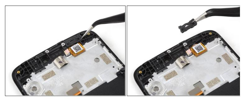
• Use a pair of tweezers to grab and remove the charging port rubber gasket.
