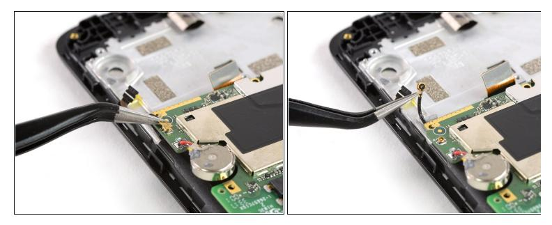
• Use a pair of tweezers to pry up and disconnect the antenna cable from the back of the motherboard.
