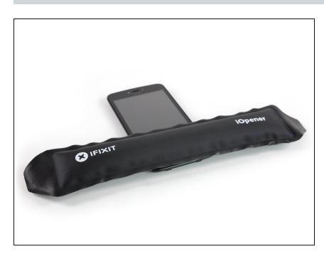
Prepare an iOpener and apply it to the bottom part of the display for at least two minutes to loosen the adhesive beneath the daughterboard.
