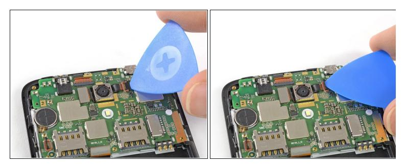
• Use the tip of an opening pick to pry up and open the black lever of the ZIF connector located at the top of the motherboard next to the rear camera.
