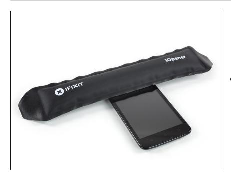
Prepare an iOpener and apply it to the upper half of the display for at least two minutes to loosen the adhesive beneath the vibration motor and the rear facing camera.
