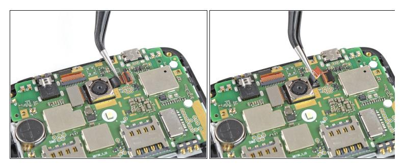
• Use a pair of tweezers to pull the digitizer flex cable out of the ZIF connector.
