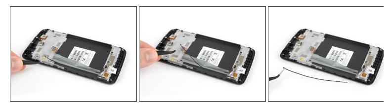
• Use a pair of tweezers to pull the antenna cable out of its routing and remove it.
