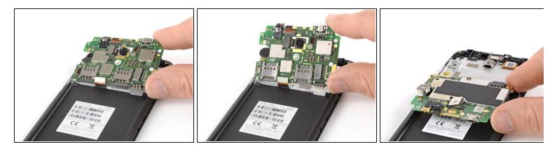
• Fold the motherboard over the battery cavity to access the coaxial cable connectors.
