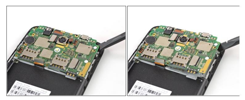
Don't try to remove the motherboard all the way yet. The antenna cable is still connected to its rear side.
