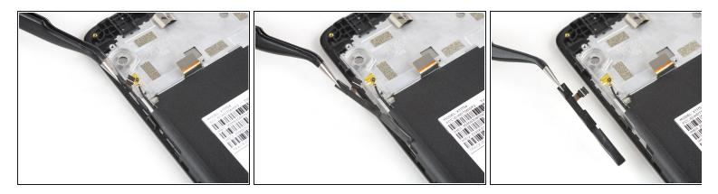
• Use a pair of tweezers to gently peel off and remove the power and volume buttons.
