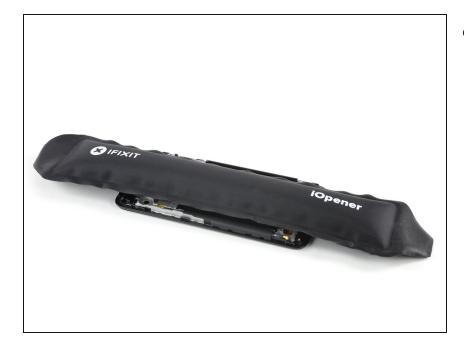
Prepare an iOpener and apply it for at least two minutes on the back of the phone to loosen the adhesive tape that sits on top of the display flex cable.
