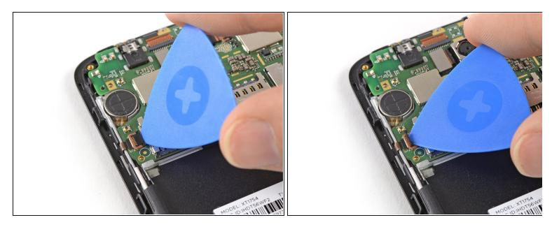
• Use the tip of an opening pick to pry up and open the black lever of the ZIF connector located on the bottom left of the motherboard.
