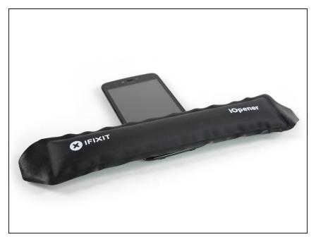
Prepare an iOpener and apply it to the bottom part of the display for at least two minutes to loosen the adhesive beneath the daughterboard.
