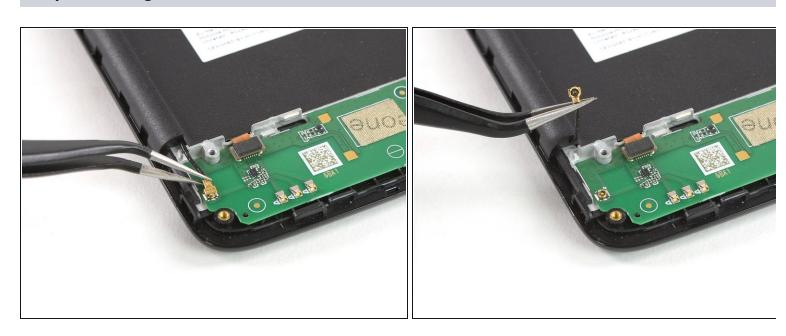
• Use a pair of tweezers to disconnect the antenna cable on the left of the daughterboard.
