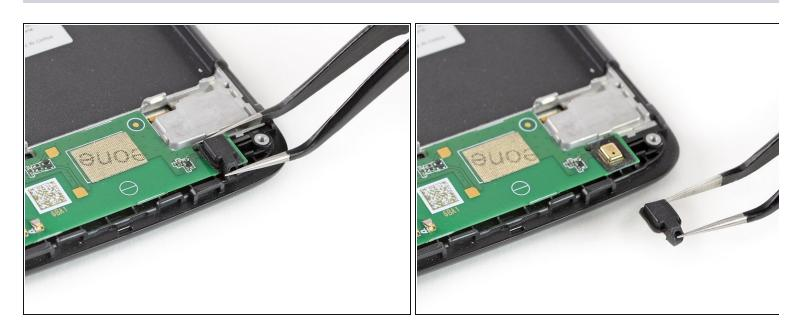
• Use a pair of tweezers to remove the rubber gasket that covers the microphone on the bottom right of the daughterboard.
