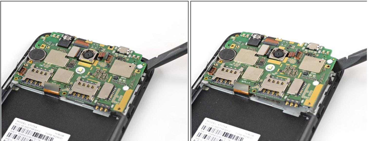
**⚠** Don't try to remove the motherboard all the way yet. The antenna cable is still connected to its rear side.
