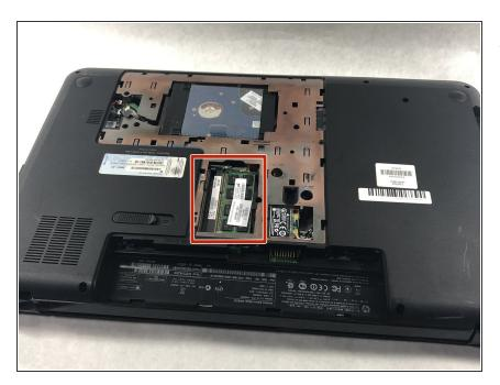
Locate the RAM modules on the device.
