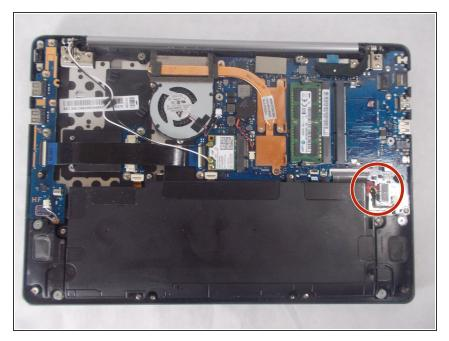
Disconnect the battery from the motherboard and remove the battery.
