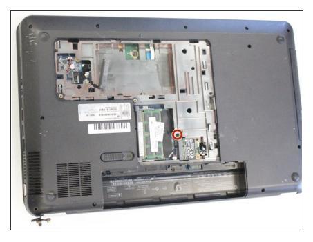
Remove the one 7 mm Phillips #1 screw securing the keyboard to the device.
