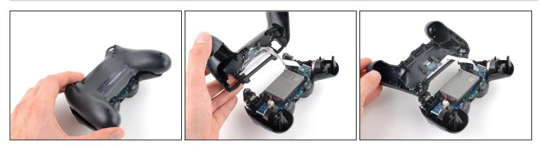
• Flip the rear case over the top of the controller and lay it down, being careful not to strain the interconnect cable.
