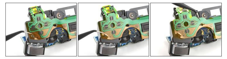
• Unclip the left half of the button circuit membrane from its two retaining pegs on the face of the midframe.
