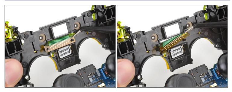
• Peel and lift the middle section of the button circuit membrane from its retaining pegs on the back of the midframe.
