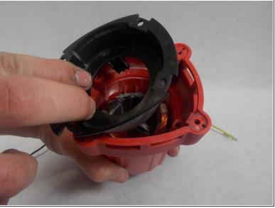
Remove the fan baffle by pulling it out.
