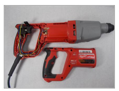
Remove the red Housing Assembly by lifting it up off of the tool.
