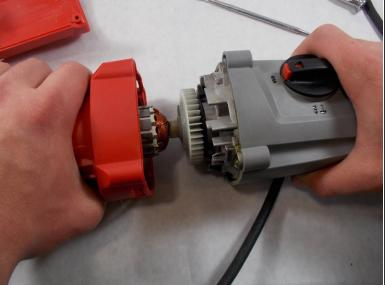
After removing the four screws, pull apart the two sections.
