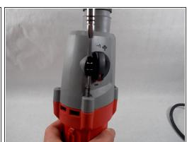
Remove the four 37mm T-20 screws shown in red. These screws attach the gear housing to the motor housing.
