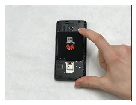
Lift up and remove the battery.
