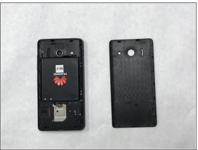
Remove the back plate by hand. There is a small indent on the bottom of the phone to pry open.
