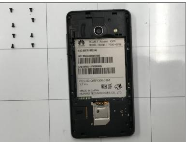
Use a T4 Torx screwdriver to remove the 8 screws along the outer edge of the case.
