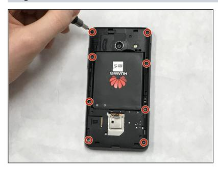
• Use a T4 Torx screwdriver to remove the eight screws.
