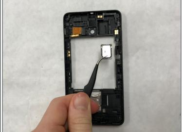
• Use the <u>tweezers</u> to remove the vibrator from the device.
