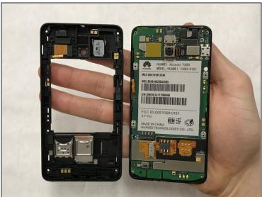
• Pry the screen from the frame by utilizing a wedge.
