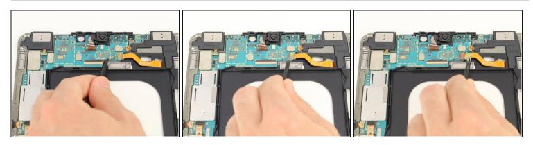
• Pull back the green tape on the upper section of the motherboard with your <u>tweezers</u> to reveal the ZIF connector below.
