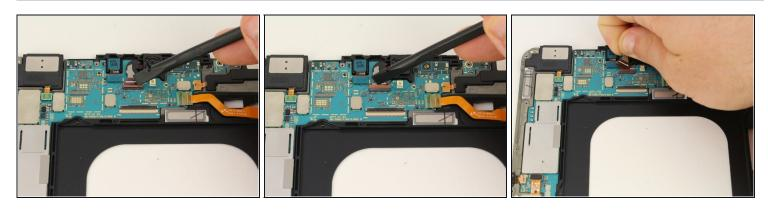
• Remove the ribbon cable for the front facing camera after popping the red ZIF connector bar up with a spudger.
