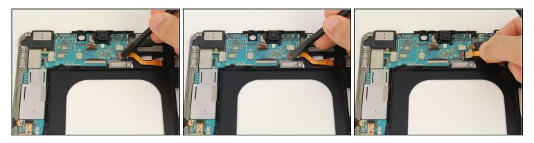
• Push the red bar up from the ZIF connector with the spudger and pull the orange, touchpad ribbon cable out.
