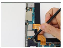
Pop the coaxial antenna cables off from the motherboard with the spudger.
