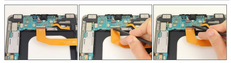
• Use the black nylon spudger to lift the gray ZIF connector up and pull out the orange ribbon cable below the camera.
