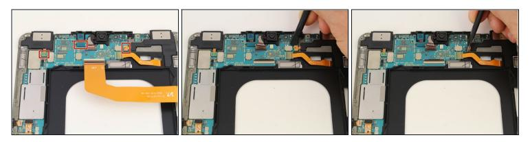
• Disconnect the three press fit connectors in the top section of the midframe by prying upwards with the spudger.
