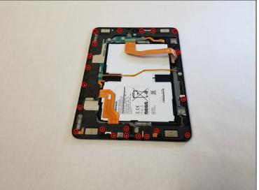
• Use a Phillips #000 screwdriver to unscrew the five screws securing the battery, and the twenty-two screws surrounding the midframe.
