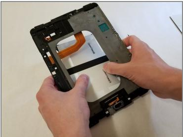
• Flip the midframe over and pop the battery out, making sure to slide it out from underneath the ribbon cables.
