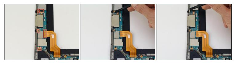
• Use the spudger to disconnect five more press fit connectors on the left side of the motherboard by prying upwards.
