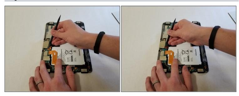
• Use the flat end of the **spudger** to pop off the connector between the battery and the motherboard.
