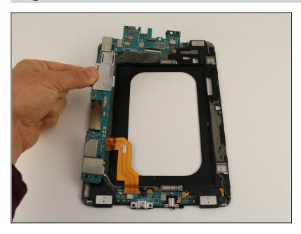
Using your fingers, move all the cables aside and wiggle the motherboard free.
