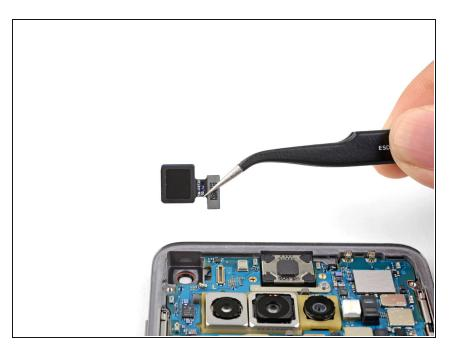
Remove the front-facing camera module. To reassemble your device, follow these instructions in reverse order.
