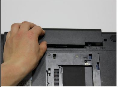
Remove the battery by pushing out the locks on either end then pushing the battery away from you.
