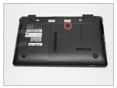
Using the J0 Japanese Industrial Standard screwdriver, remove the 4.5mm screw on the ODD/HDD Memory panel.
