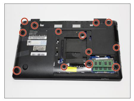
Using the J1 Japanese Industrial Standard screwdriver, remove the thirteen 9.5mm screws from the panel that cover the bottom of the computer.
