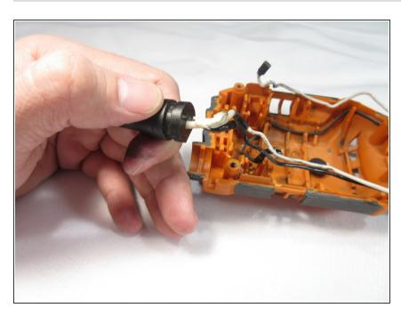
Lift the cord up and out of the device.
