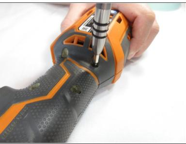
Completely remove all eight 15mm T10 Torx screws.
