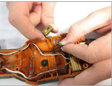
Firmly hold the brush in one hand and pull at the base of the wire to disconnect.
