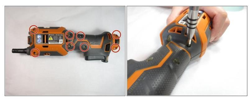
Completely remove all eight 15mm T10 Torx screws.
