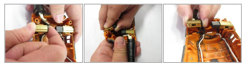
• Pinch the brush and pry upward away from the center of the part to remove from the device.
