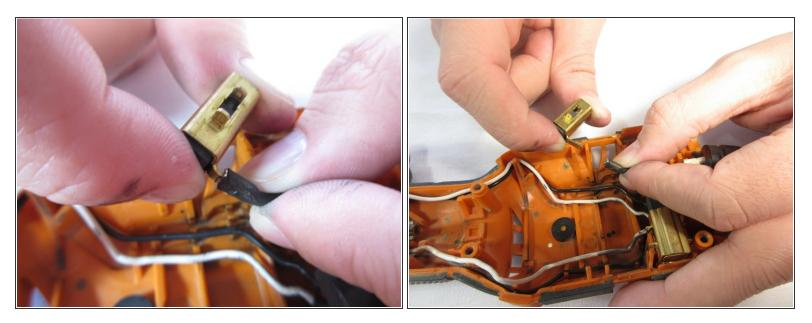
• Firmly hold the brush in one hand and pull at the base of the wire to disconnect.
