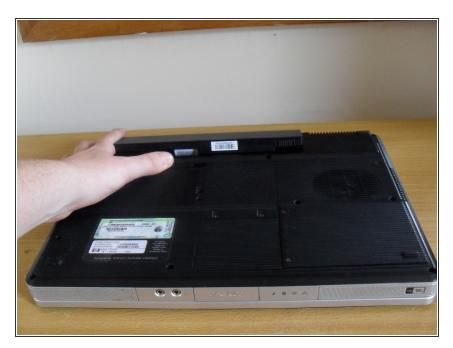
Start by removing the battery
