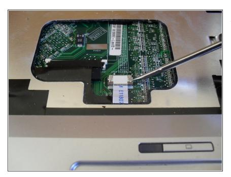
Use a flat blade screwdriver to loosen the touchpad cable connecter
