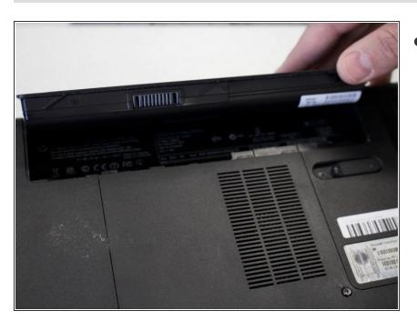
Lift and remove the battery from its compartment.
