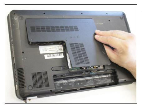
Slide the service panel down and pull it up to remove.
