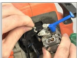
Detach the throttle cable from the carburetor by tilting it 90 degrees and pulling up.
