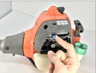
Slide the choke lever to the full choke position.
