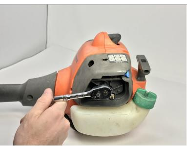
Remove two 8mm nuts with an 8mm socket attached to a 1/4" ratchet turning the nuts counterclockwise.
