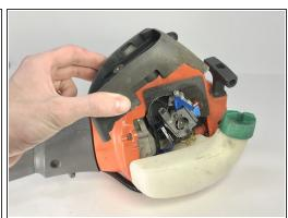
Remove the plastic housing by pulling it away from the device.
