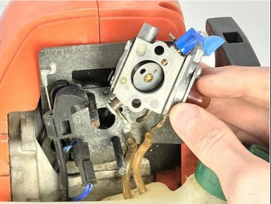
Remove the two fuel lines attached to the bottom of the carburetor using a set of needle nose pliers.
